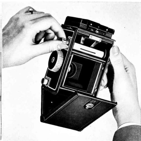
Inserting the empty film spool in- to the take-up chamber
